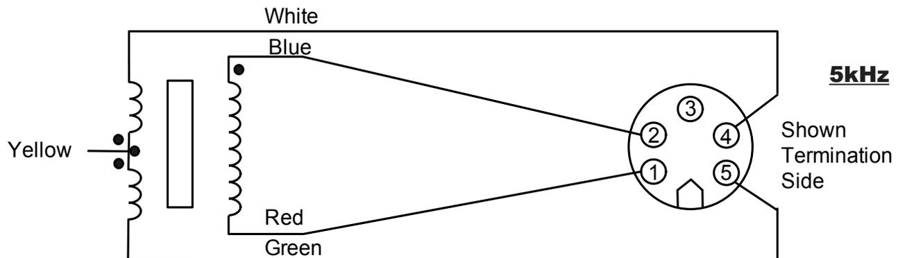
**Figure 3 Connector Terminations - 5kHz**
